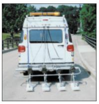
Investigators performing nondestructive testing on concrete pavements are mobile now thanks to the innovations in using easy-totransport radar sending, receiving, and data-recording units. makes it easier to transport the system.
