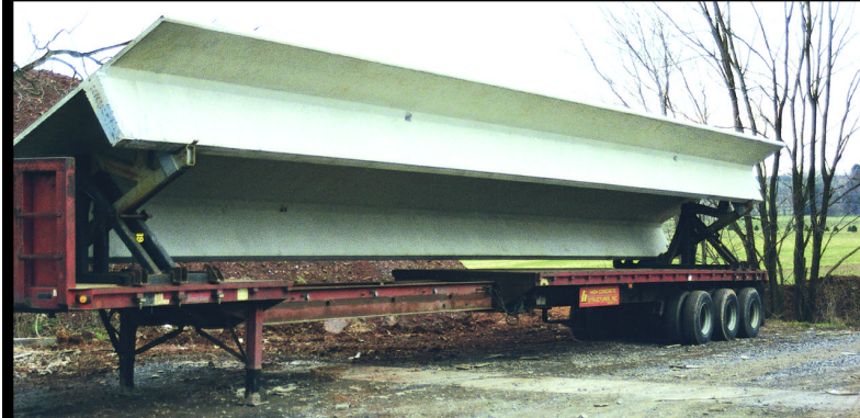
If you've ever carried a couch through a doorway, you know how High Concrete Structures' new invention for tilting large structural concrete pieces works. The "Loading Fixture" reduces load width by tilting pieces at an angle.
