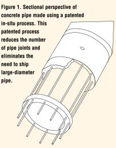
inner and outer surface of the pipe. These alternative forms provide convex nesting embers. In turn, these embers form internal conduits between the inner and outer surfaces that accept reinforcing members or connection members to interlock the forms together. Concrete fills in these conduits and between the void of
