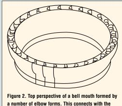
a number of elbow forms. This connects with the end of an adjacent pipe.
